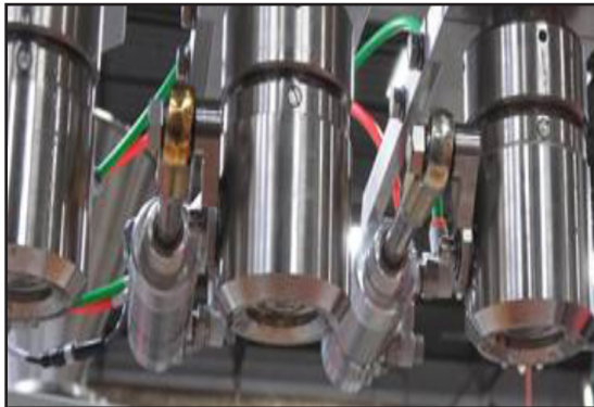
Pneumatic actuators on filling machine.
